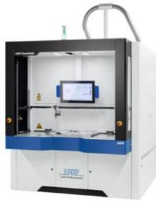
**Figure 3:** An LPKF laser machine, comparable to this LPKF PowerWeld 6600 model, welds the valve block components together.
