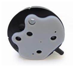
**Figure 2:** One of the key components of the device: The valve block consists of a laser-transparent and a laser-absorbing plastic element - firmly welded and tested for pressures up to 400 bar.
